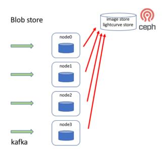
The next stage of the prototype is to treat binary data (images, perhaps also lightcurves) in the same way as the database records. The cache will be the local file storage, then when the data flow stops, transferring these to the blob store. Parallel Ingestion and Workflow - Andy Lawrence - LSST:UK
