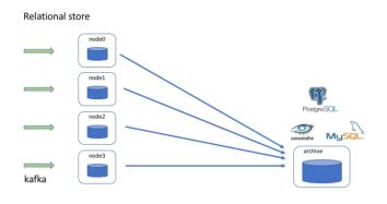
The ingestion nodes and archive node are shown here. The nodes share the kafka stream of alerts, coming in from the left, and they build a database record corresponding to each alert, which they write to a cache, a node-local database. Thus all the nodes work in parallel with no serial
