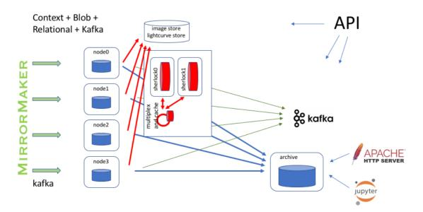
Here are all the moving parts of the system, an architecture that implements the required functionality. Services are set up and waiting, then each node starts consuming Kafka from the MIrrormaker cache. While 4 nodes are shown, it could be any number to achieve sufficient speed. Similarly with the sherlock cluster. Consumers can use the website to build complex filters, they can also use the Jupyter interface, consume a Kafka stream, or code against the Lasair API.
