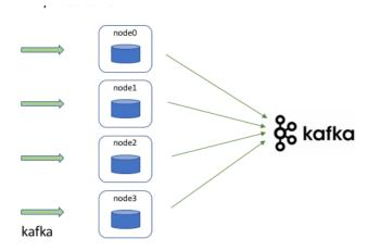
A kafka producer can be added to each node. All the user-built queries will be available to each node, and all of them run against the alerts that the node has, and when the query is successful, the output matrixed together by a kafka producer node.
