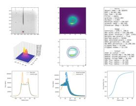
100Hz), so it can be seen if there is stiction, wind shake, etc. Basically, if those are smooth you know your PSF is going to be OK, modulo focus etc. This plot is made for all images for which the telescope is tracking, and the exposure time is 2s.
