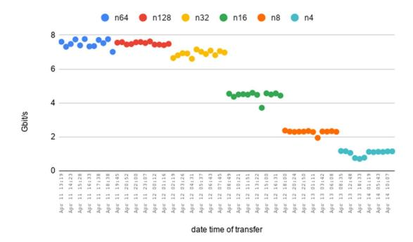
The highest transfer speeds achieved, **7.5 Gbit/s**, are close to saturating the bandwidth of the local, 10 Gbit/s, network switch.
